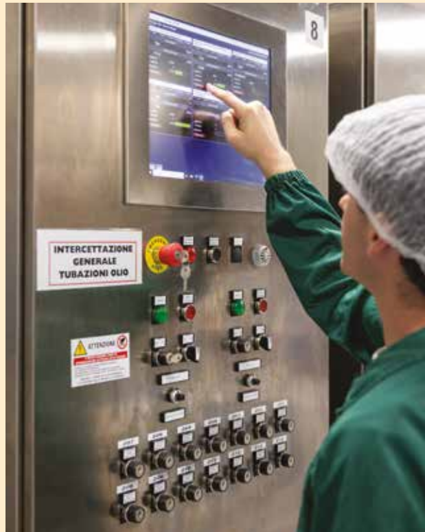
An integrated management and control system for oil discharge, storage and handling of bulk/unbottled oil
